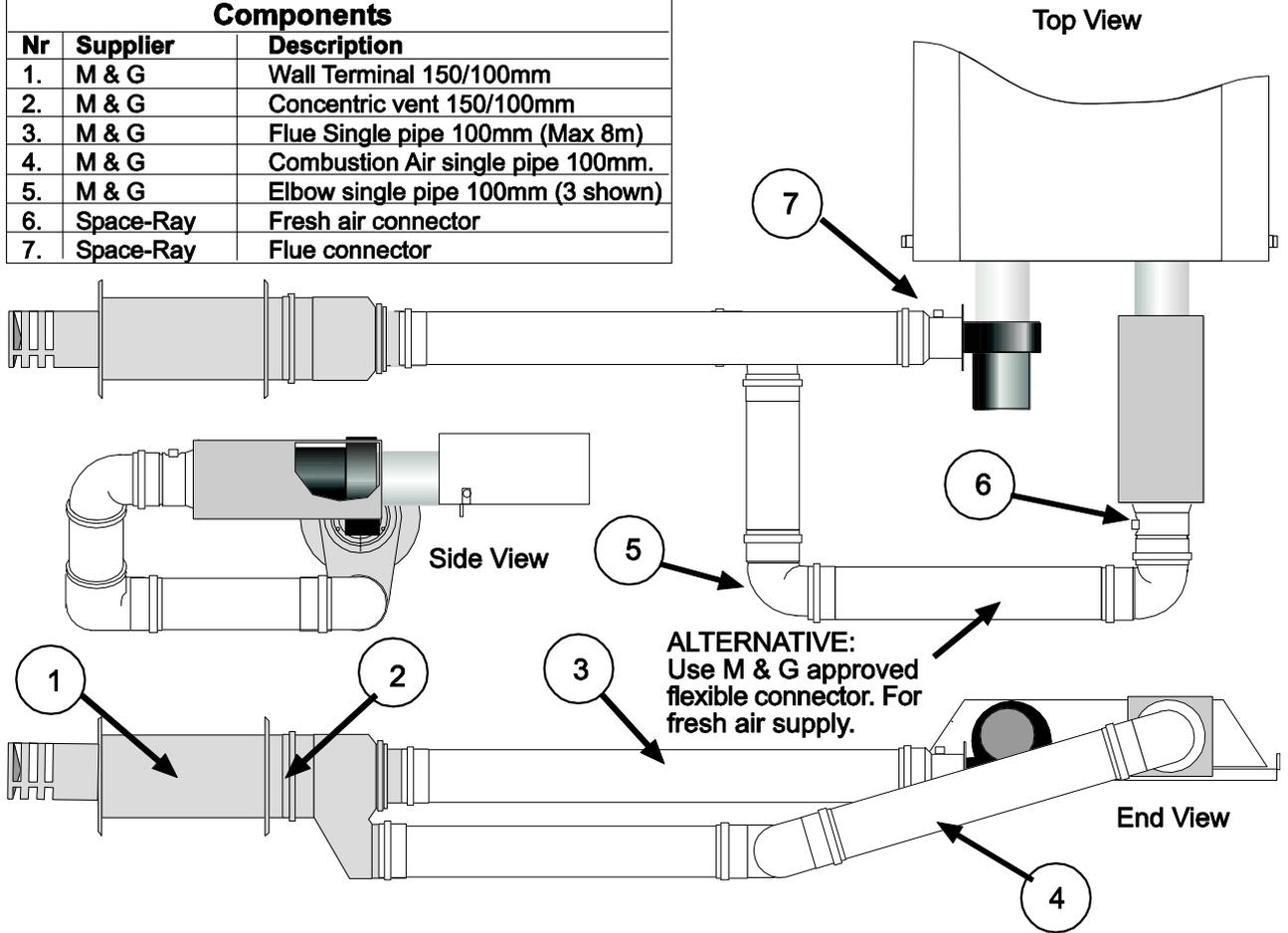
Above shows typical arrangement for flue to the side of the heater
