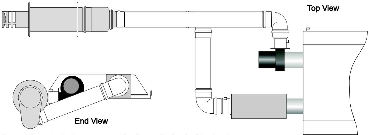
Above shows typical arrangement for flue to the back of the heater
