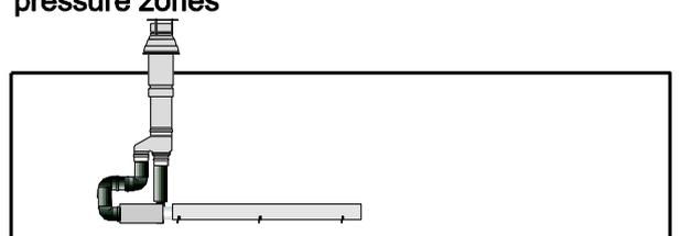
C32 - Fresh air & Flue vertical in concentric ducts
