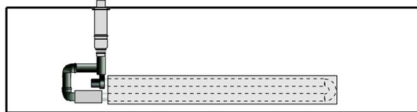
C12 - Fresh air & Flue horizontal in concentric ducts
